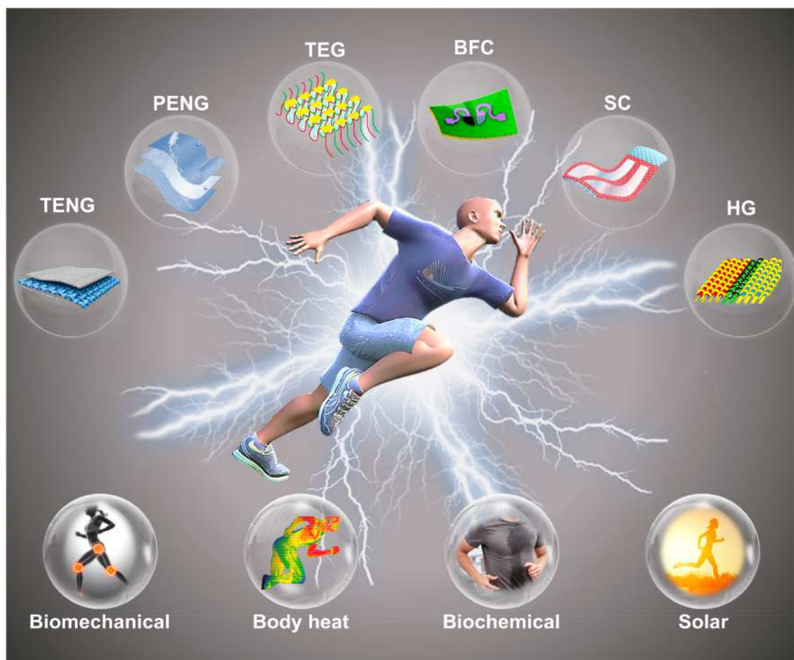
Figure 1. Schematic illustration of smart textiles for energy harvesting. The human body and its surroundings, including biomechanical motions, body heat, biofluids, and sunshine, are rich sources of renewable energy. Fusion of textiles and generators to generate electricity from the human body and its ambient environment renders a pervasive, environmentally friendly, and sustainable energy solution for wearable electronics in the era of the Internet of Things.
